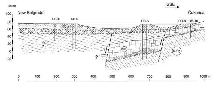
Fig. 7. A simplified geological cross-section along the route of the new bridge. Key: K-Pg, Upper Cretaceous-Paleogene; Sm, Middle Miocene Sarmatian; Pn, Upper Miocene Pannonian;  $Q_1$ , Pleistocene,  $Q_2$ , Holocene.  $\sqrt{-Assumed}$  fault.
