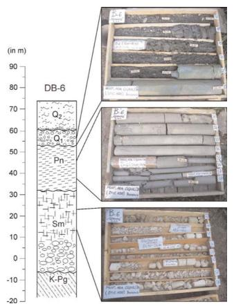
Fig. 3. The stratigraphic column and the core samples from the borehole DB-6. For the key, see Fig. 2.
