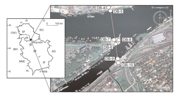
Fig. 1. The projected position of the new bridge over the Ada Ciganlija Island (Belgrade) and the locations of the investigated boreholes (Google Earth, 2011).
