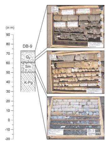
Fig. 2. The stratigraphic column and the core samples from the borehole DB-9. Key: **K-Pg**, Upper Cretaceous–Paleogene; **Sm**, Middle Miocene Sarmatian; **Pn**, Upper Miocene Pannonian;  $Q_1$ , Pleistocene,  $Q_2$ , Holocene.
