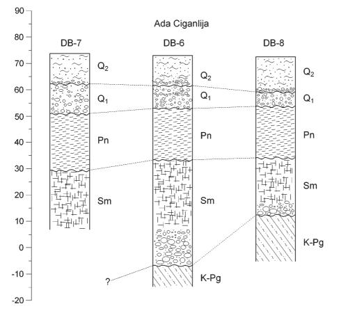
Fig. 5. Comparative stratigraphic sections of the boreholes at the tip of Ada Ciganlija. For the key, see Fig. 2.
