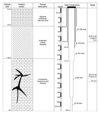
Fig. 3. Lithological profile and construction of well B-2 (after MILOJEVIĆ, 1973, simplified).
