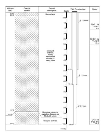
Fig. 2. Lithological profile and construction of well B-1 (after MILOJEVIĆ, 1973, simplified).
