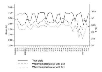
Fig. 4. Flow rates and water temperatures of the wells B-1 and B-2 (August 2000 – February 2002).
