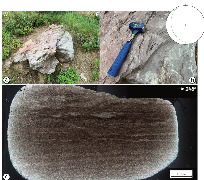
Fig. 3. An example of structural – geological mapping at observation point 23J002. a) Oriented photo of an outcrop; b) Photo of oriented sample for further microtectonic study, with a structural diagram showing the principal foliation plane; and c) photomicrograph of oriented sample 23J002.
